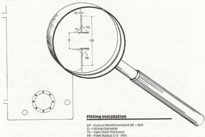
TO—Outside Installation Laminate Thickness TI—Inside Installation Laminate Thickness Another area of interest is the minimum physical property requirements for fiberglass laminates at various thicknesses. The following table gives minimum acceptable physical properties in three important areas.
