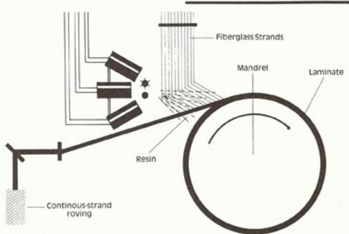
Filament winding can be and is commonly combined with the chop spray method. By combining the two processes a monolythic tank wall with superior strength and liquid retention capabilities can be produced.
