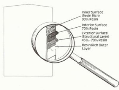
The Interior layer comes next and is included to back-up and reinforce the inner surface. A ratio of 70% resin to 30% fiberglass is desirable and is most commonly applied using the chop spray method. This layer should be applied in two or more passes and in combination with the inner liner, be a minimum of .100 inches thick. Unlike the C-Veil or Nexus inner liner, it is difficult to determine if a good interior layer has been applied, unless sophisticated equipment is available for testing.
